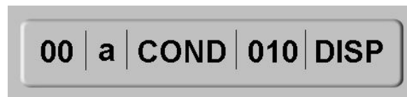
Fig. 2. Branch instruction format for the Sparc processor family.
